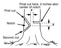
Hinge holds tree on stump and helps control fall
